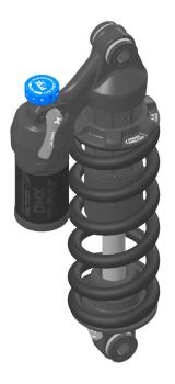
The **Low-Speed Compression knob** allows for changes in low-speed compression damping. Turn the knob clockwise to increase compression damping and counterclockwise to decrease compression damping.
